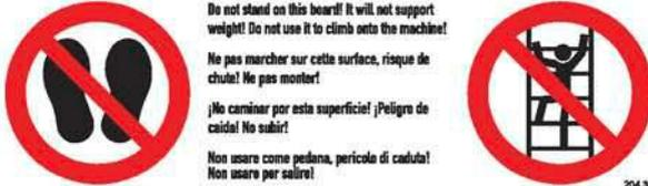
Do not stand on this board! It will not support weight! Do not use it to climb onto the machine!
